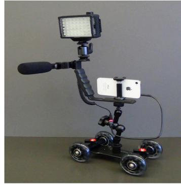
Figure 2: Smartphone dolly with external microphone and lighting.
